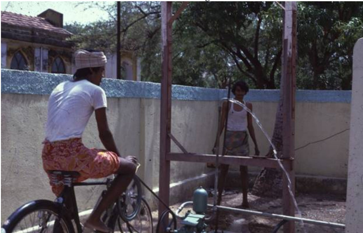
Water Pumping from a Shallow Well
